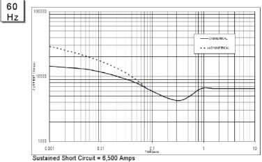
1.The following multiplication factors should be used to adjust the values from curve between time 0.001 seconds and the minimum current point in respect of  $\underline{\text{nominal operating voltage}}$
