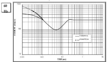
1.The following mult Sustained Short Circuit = 240 Amps point in respect of nominal operating stronger
